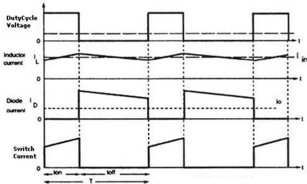
Figure 9.2: Boost Converter Waveforms
