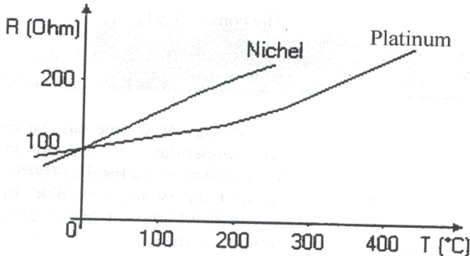
Normally used RTD's have a resistance of  $100 \Omega$  at  $0^{\circ}\text{C}$  and a tolerance of  $(\pm 0.1)^{\circ}\text{C}$ . They usually consist of a wire of the above materials wound around a cylindrical insulating material or a plate resistant to high temperatures (ceramic, glass). For their constitution, as they have a very high thermal constant, they are relatively slow in following the process temperature variations.
