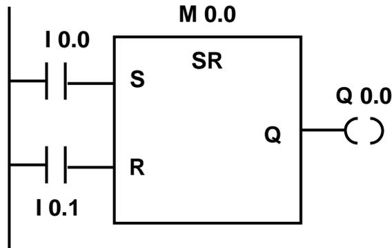
If the signal state is "1" at input I0.0 and "0" at I0.1, memory bit M0.0 is set and output Q0.0 is "1". Otherwise, if the signal state at input I0.0 is "0" and at I0.1 is "1", memory bit M0.0 is reset and output Q0.0 is "0". If both signal states are "0", nothing is changed. If both signal states are "1", the reset instruction dominates because of the order; M0.0 is reset and Q0.0 is "0".
