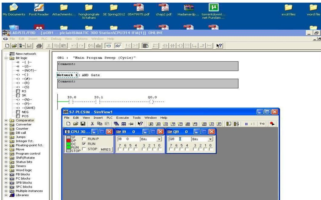
15. Select bit for Logic 1 and unselect for Logic 0. Verify the AND logic.
