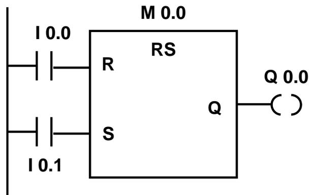
If the signal state is "1" at input I0.0 and "0" at I0.1, memory bit M0.0 is set and output Q0.0 is "0". Otherwise, if the signal state at input I0.0 is "0" and at I0.1 is "1", memory bit M0.0 is reset and output Q0.0 is "1". If both signal states are "0", nothing is changed. If both signal states are "1", the set instruction dominates because of the order; M0.0 is set and Q0.0 is "1".
