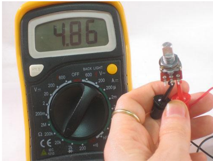
Potentiometer centered, about 5K\Omega
