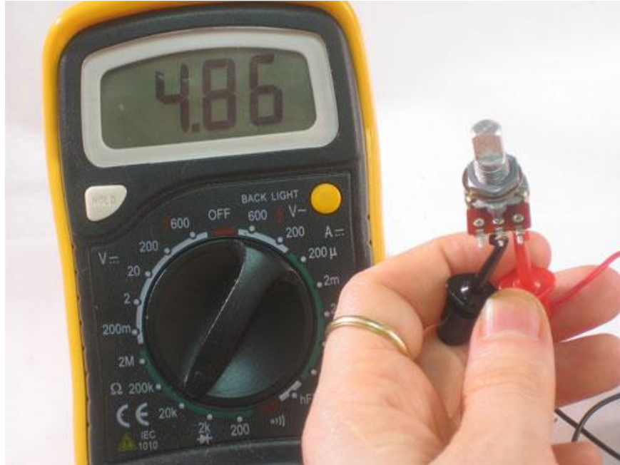
Potentiometer centered, about 5K
