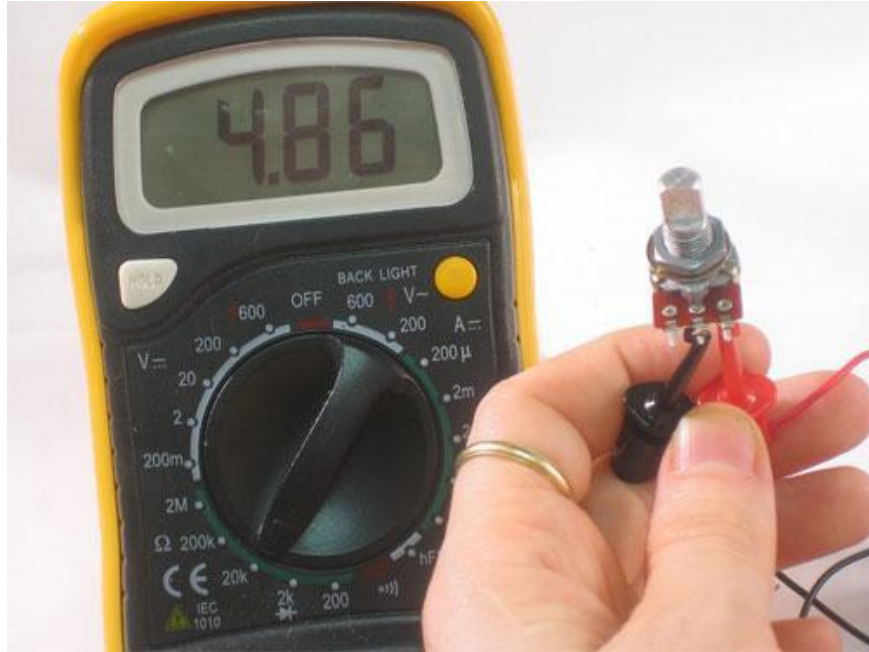
Potentiometer centered, about 5K\Omega
