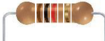
This image shows a 1.0 k \Omega 5% resistor (brown black red gold)
