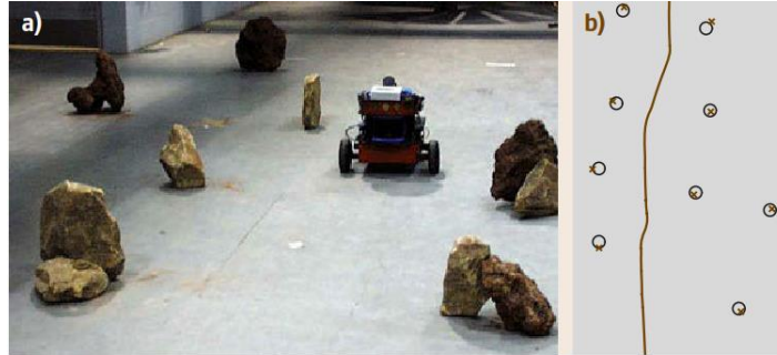
A mobile robot scanning the environment and generate landmark based map
