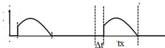
Figure 3.6: Measuring tx and \Delta t for Single Phase Halfwave Controlled Rectifier
