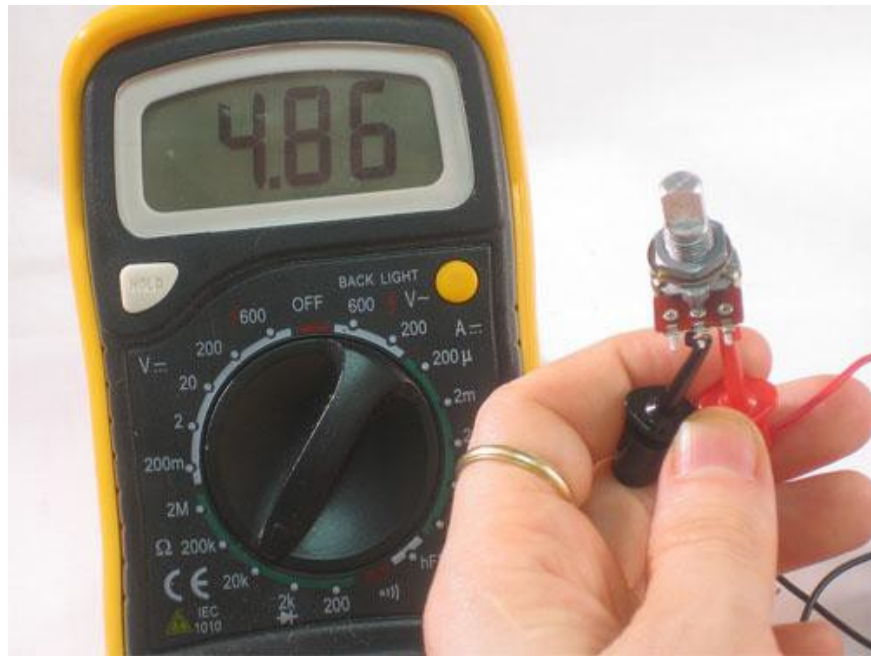
Potentiometer centered, about 5\text{K}\Omega
