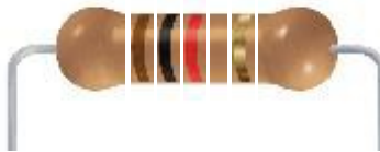
This image shows a 1.0 k \Omega 5% resistor (brown black red gold)
